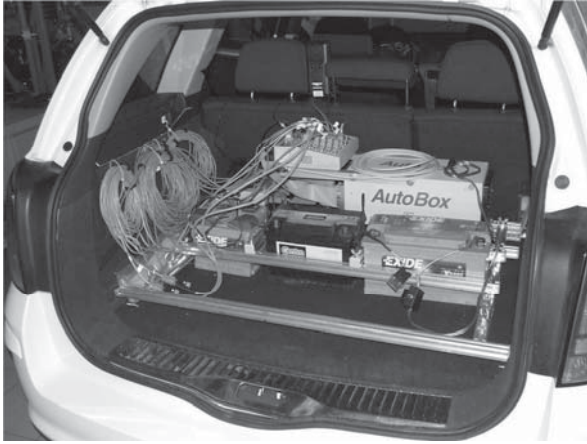
Fig. 1. The view of some hardware used to implement a prototype suspension controller inside test vehicle
