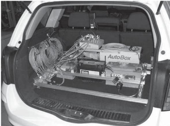
**Fig. 1.** The view of some hardware used to implement the prototype suspension controller inside test vehicle
