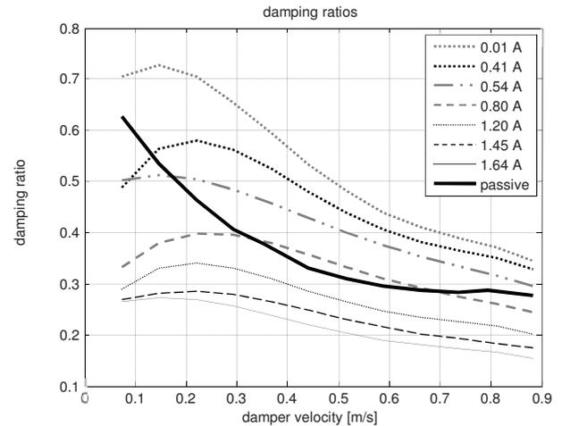
**Fig. 2.** Damping ratios of the passive and semi-active suspension of investigated vehicle with sprung mass corresponding to curb vehicle weight
