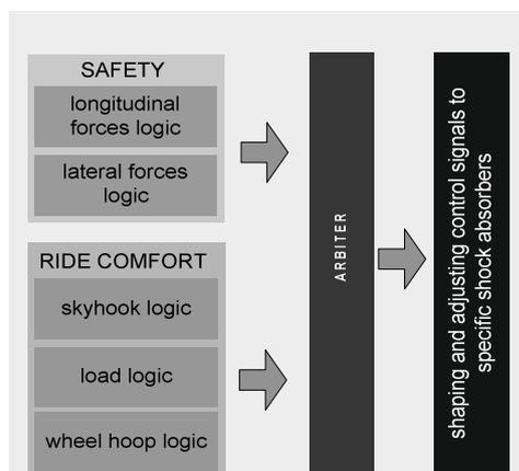
Fig. 4. Suspension controller module architecture diagram
