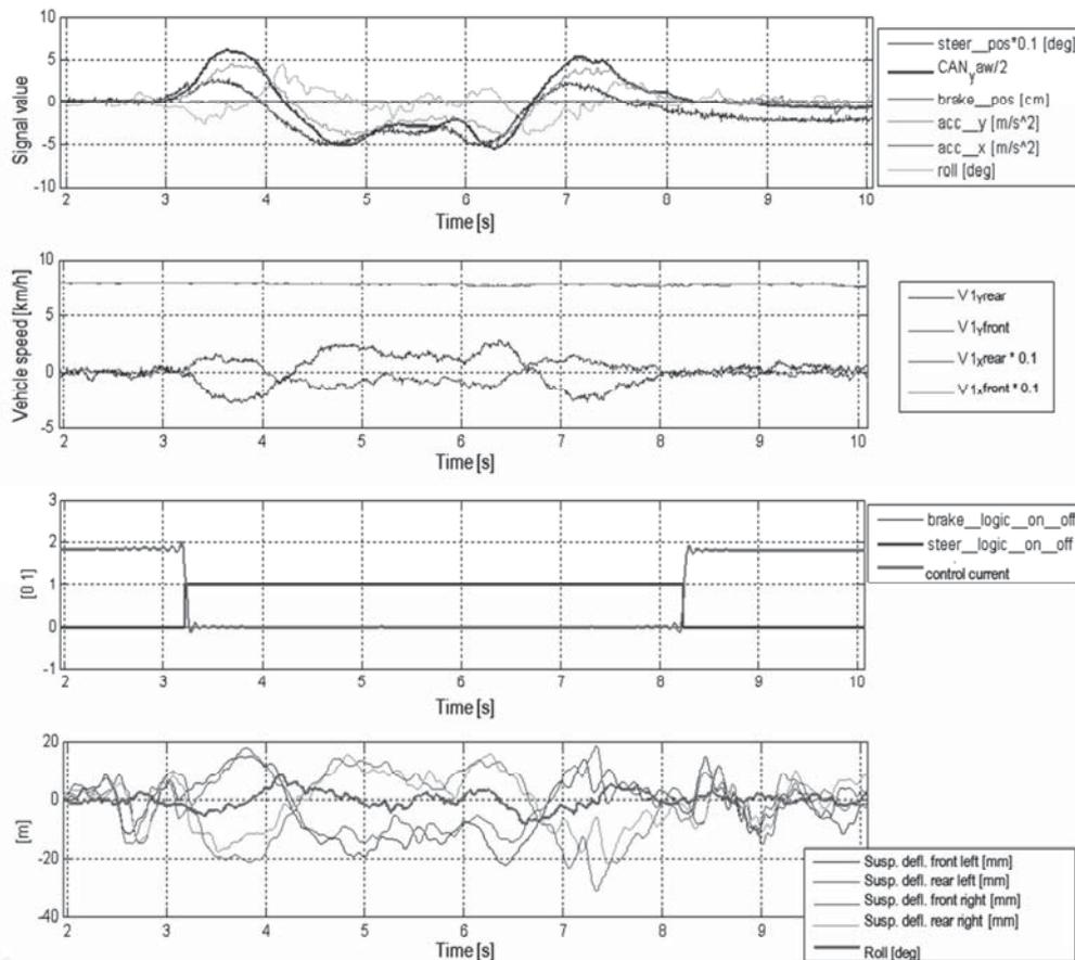
Fig. 6. Results of measurements made during drives through ISO 3888-1 track
