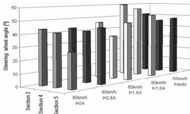
Fig. 7. Steering wheel angle peak values comparison for various test drives of ISO 3888-1 test
