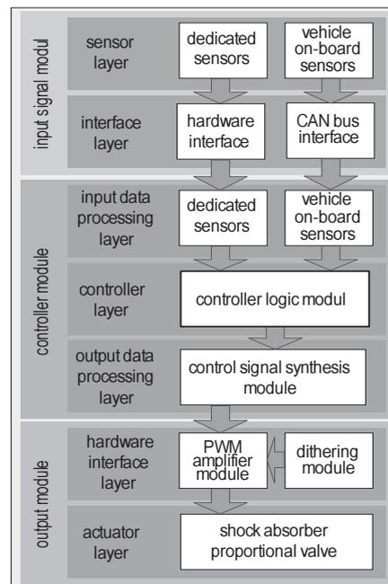
**Fig. 3.** Suspension controller architecture diagram
