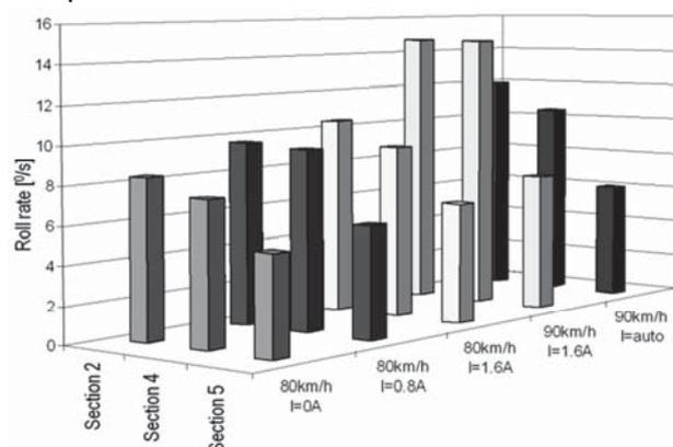
Fig. 9. Roll rate peak values comparison for various test drives of ISO 3888-1 test
