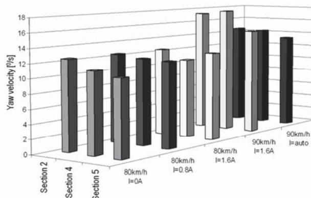
Fig. 8. Yaw velocities peak values comparison for various test drives of ISO 3888-1 test
